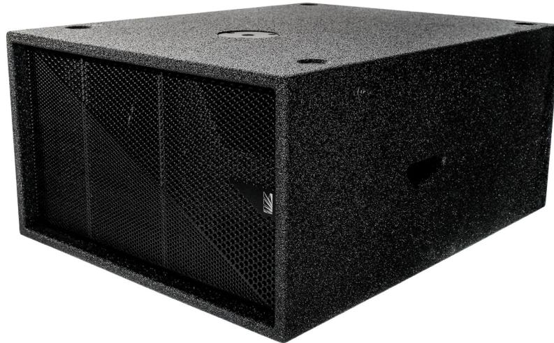
The Harrier Dub 12 is a low frequency loudspeaker featuring a pair of 12" (320mm) transducers with a 4" (100mm) voice coil. Drivers are slot loaded and aligned in a push pull configuration to reduce distortion.
