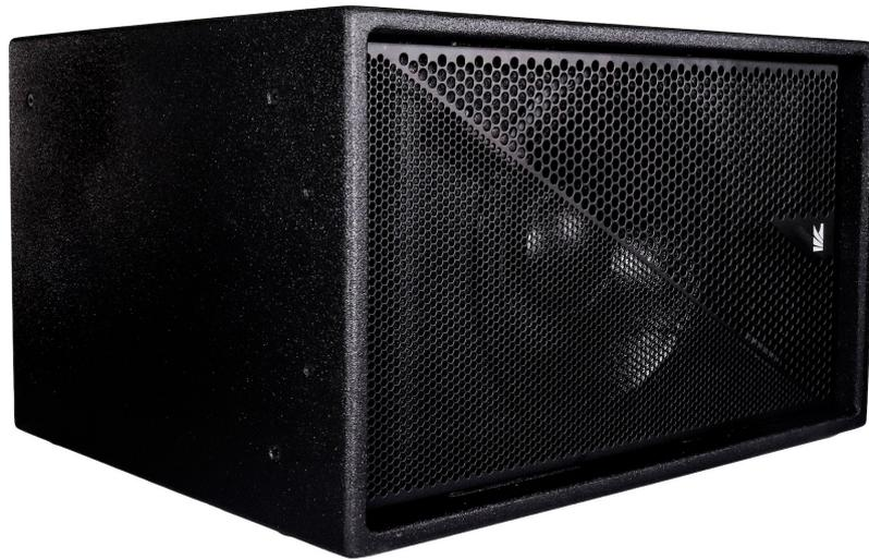
The Hawk Solo 12 is a low frequency loudspeaker featuring a 12" (320mm) transducer with a 3" (76mm) voice coil. It has a large flared port to give laminar flow and maximize acoustic output.
